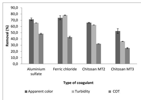
**Figure 1.** Percentage of removal of the optimal dosage of each coagulant; Aluminum sulfate (40 mg/L), ferric chloride (60 mg/L), Chitosan MT2 (5 mg/L) and MT3 Chitosan (10 mg/L). **Table 2.** Results of the analyzes performed for each coagulant at different doses
