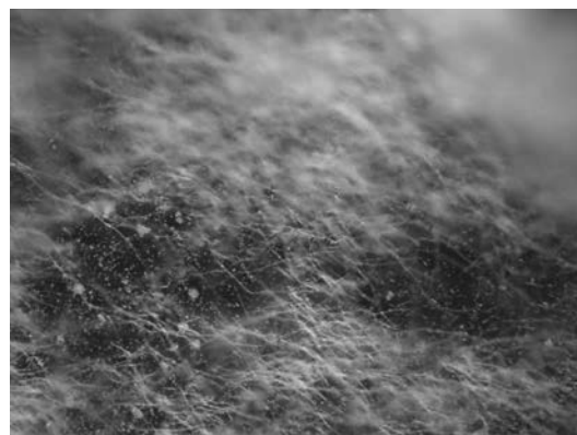
Figure 4. Immobilized A. niger on glass coupons.
