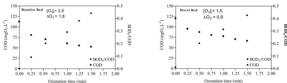
**Figure 4:** Change of biodegradability index ( $BOD_5/COD$ ) and COD with time during the ozonation of direct and reactive red dyes;  $[Dye]_{i=0}$  50 ppm, Temperature = 15 °C and  $pH = 5.1 \pm 0.1$ .
