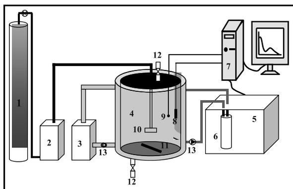
(1)-O<sub>2</sub> Cylinder (2)-O<sub>3</sub> Generator (3)-Water thermostat (4)-Reactor (5)-UV-vis. Detector (6)-Flow Cell (7)-Data Acquisition (8)-pH meter (9)-Thermometer (10)-O<sub>3</sub> Diffuser (11)-Magnetic stirrer (12)-ports (13)-Circulating pumps
