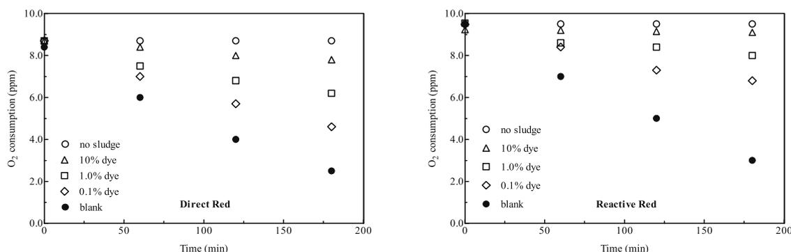
Figure 2: Inhibition of O<sub>2</sub> consumption by activated sludge for untreated dye solutions (Initial concentration=50 ppm, Temperature = 15 °C and pH= 7.0± 0.2).
