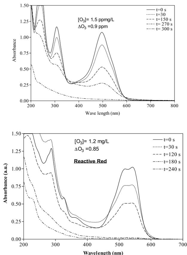
**Figure 3:** Spectral changes with time during the ozonation of direct and reactive red dyes; [dye]<sub>i</sub>=50 ppm, Temperature = 15 °C and pH = 5.1 ± 0.1
