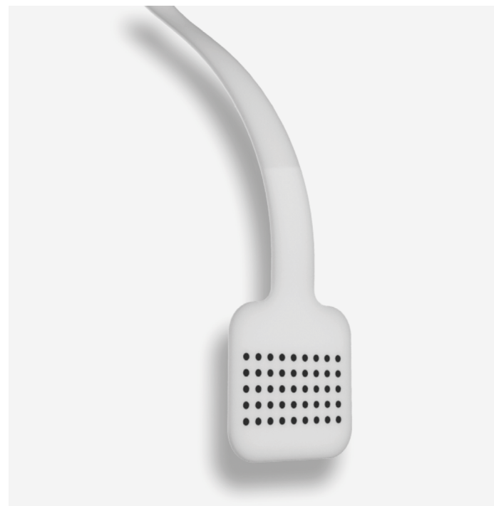
Fig. 13. The BrainPort V100 oral electronic vision aid, produced and approved by the Food and Drug Administration (FDA) in 2015.
