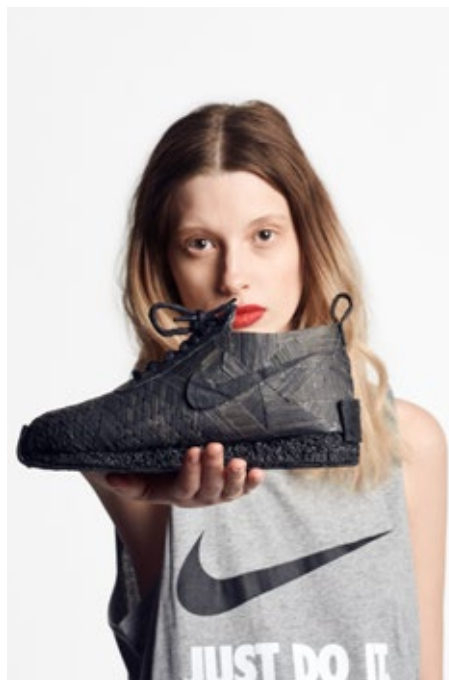
Fig 2. Image of the process and the final prototype. This participant worked with wood processed as fibres and shavings and mixed with natural rubber. The materials created show excellent properties and received very positive feedback from the designers in the collaborating company. However, the material would need to be developed further to be durable enough for a shoe. Also, because of this apparent incompatibility between material and the functionality of the product, the shoe decreases the perceived value of the material to some degree. (Trial 4)
