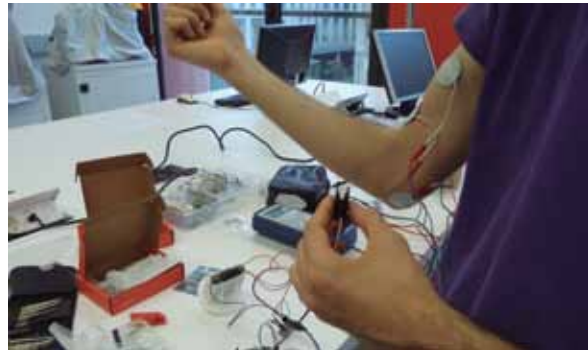
▼ Figure 16. Control of the servo motor that generates movement of a finger triggered by electromyographic signals from muscle contraction and relaxation.
