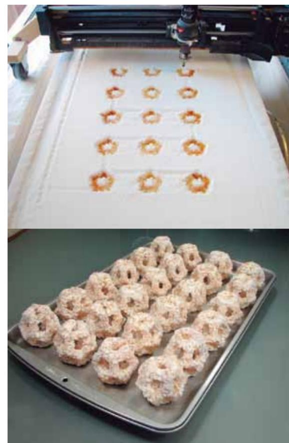
▲ Manufacturing process with an experimental machine where the raw material is sugar. CandyFab 4000 by Evil Mad Scientist Laboratories.
