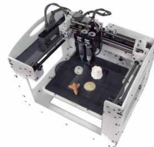
▲ Fab@Home Model 2 3D printer and printed parts. Hod Lipson
