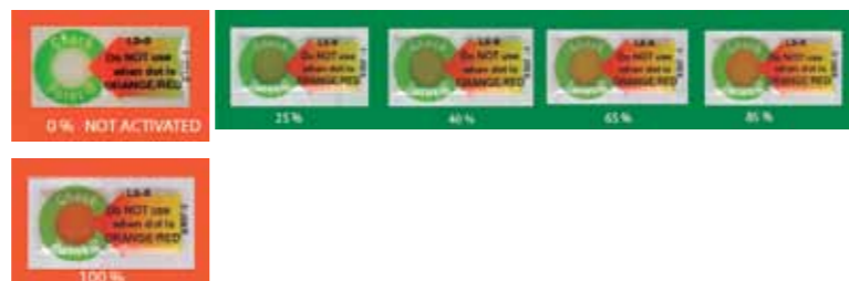
▲ 3. The VisaLab label distinguishes between the inactivated state, in which the product is fit for consumption, and the activated state, when it is not deemed safe. < http://vitsab.com/index.php/tti-label/ >
