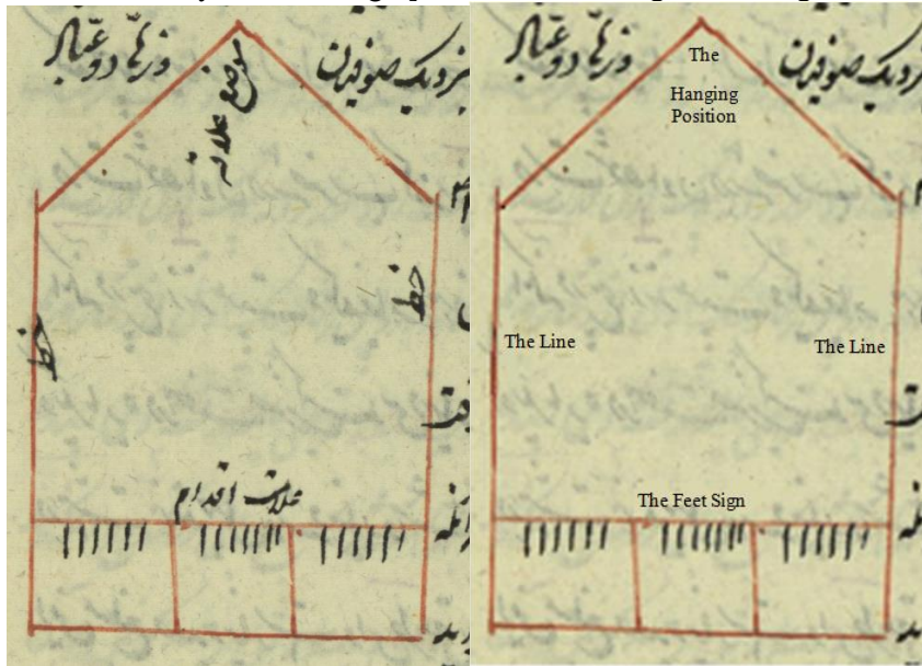
[Fig. 1. A kind of gnomon which was used for determining the 'aṣr prayer time by Muslims ( Yawāqīt al-'Ulūm wa Darārī al-Nujūm , ms. preserved in Loghatnameh Dekhoda Institute, no. 95, f. 64 r)]
