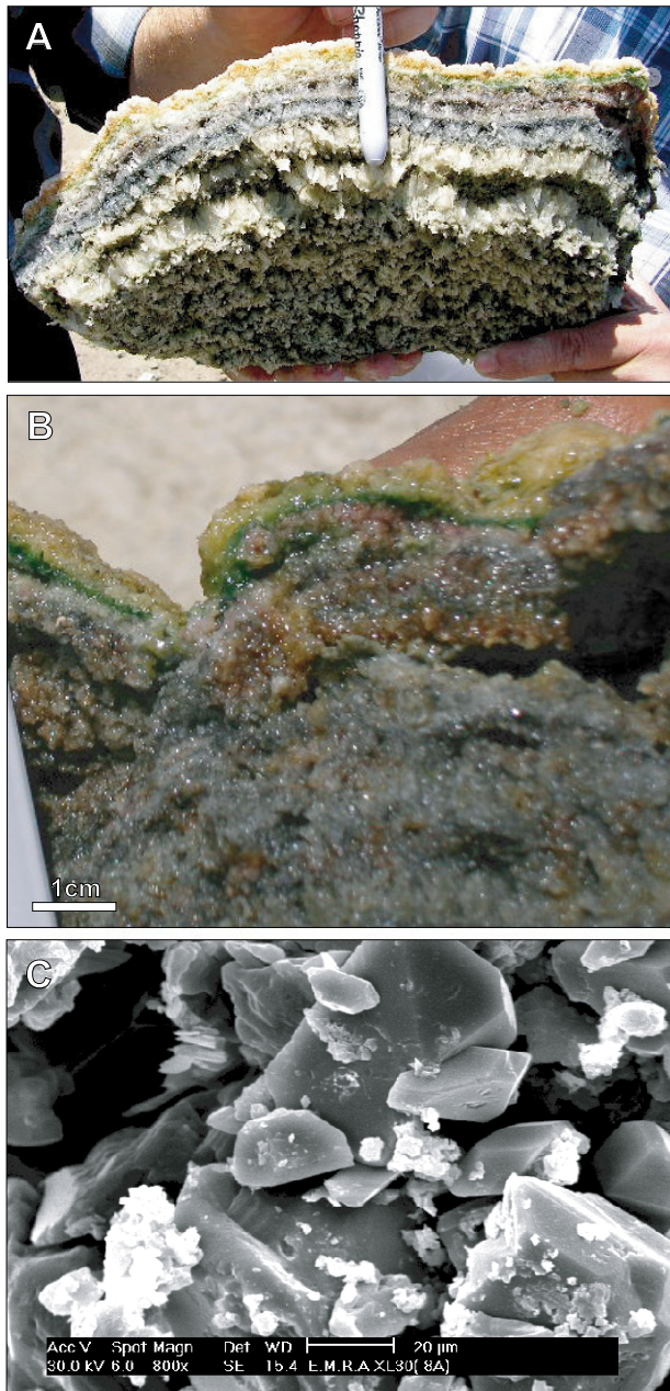
FIGURE 5 | A) Laminated selenite (grass-like subfacies). B) Fine grained gypsum microbialite (stromatolite) subfacies. C) SEM micrograph of fine lenticular gypsum crystals embedded in microbial biofilm (gypsum microbialite).
