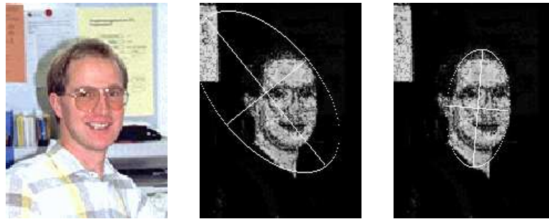
Figure 4: First: the original input image. Second: the Global Fit Ellipse (GFE) on the skin map. Third: the Local Fit Ellipse (LFE) on the skin map
