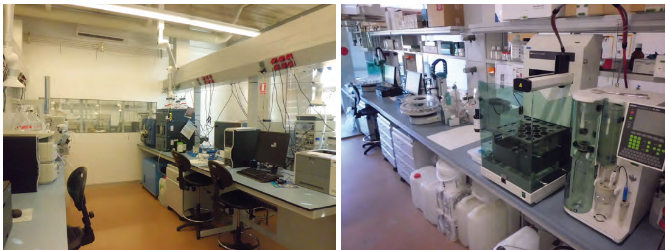
Fig. 3. View of the Scientific and Technical Services (SCT) facilities at ICRA, showing the GC/MS and LC/MS equipment (left) and the Chemical Analysis Unit (right).
