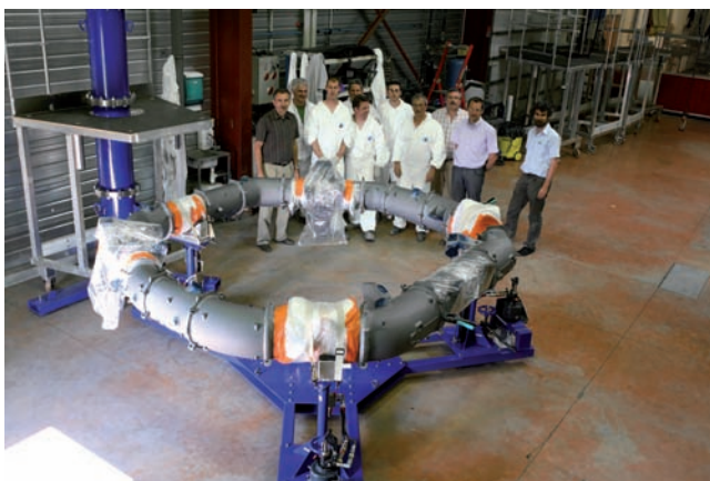
Fig. 6. Members of the BOOSTEC and Astrium team just after the torus removal from the brazing furnace. The torus is made of SiC and consists of 16 different pieces independently manufactured. (Courtesy of ESA).
