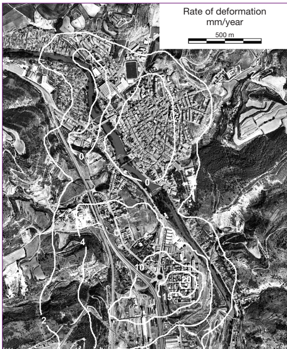
Figure 4 Average rate of vertical deformation of the land in the area of Sallent (Bages), estimated with the DInSAR technique over a period of five years.
