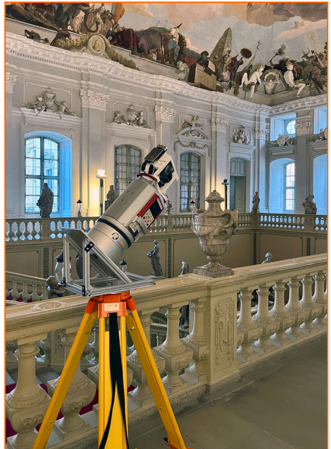
Figure 2. Pulsed laser scanner Riegl VZ-400, part of the multimodal real-time scanning unit Irma3D, on the Würzburg Residenz's monumental staircase. Source: Paolo Patelli
