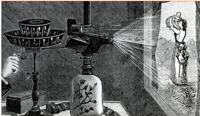
Figure 13. Reynaud's Projection Praxinoscope Source: La Nature, Revue des Sciences, 1882
