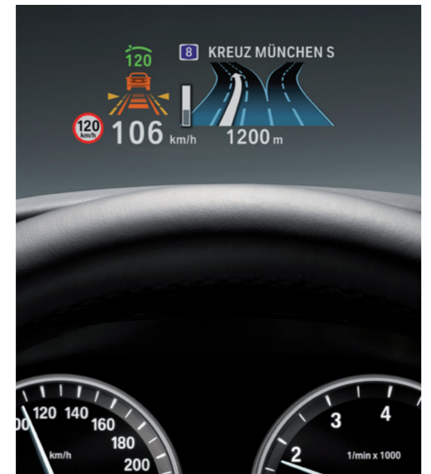
▼ Image 3. New head-up display with enhanced navigation systems. Photo: BMW AG.
